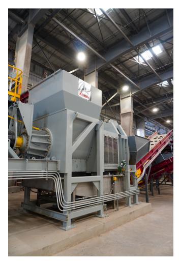
The OSP separates and recovers organics liquid for transport to anaerobic digestion facilities. There, the organic pulp is converted to renewable gas that can be used to fuel Athens' collection fleet. The process also diverts methane-producing material from landfills. Both steps will help Athens customers and cities to comply with California's climate initiative programs to reduce greenhouse gases, such as SB 1383.
